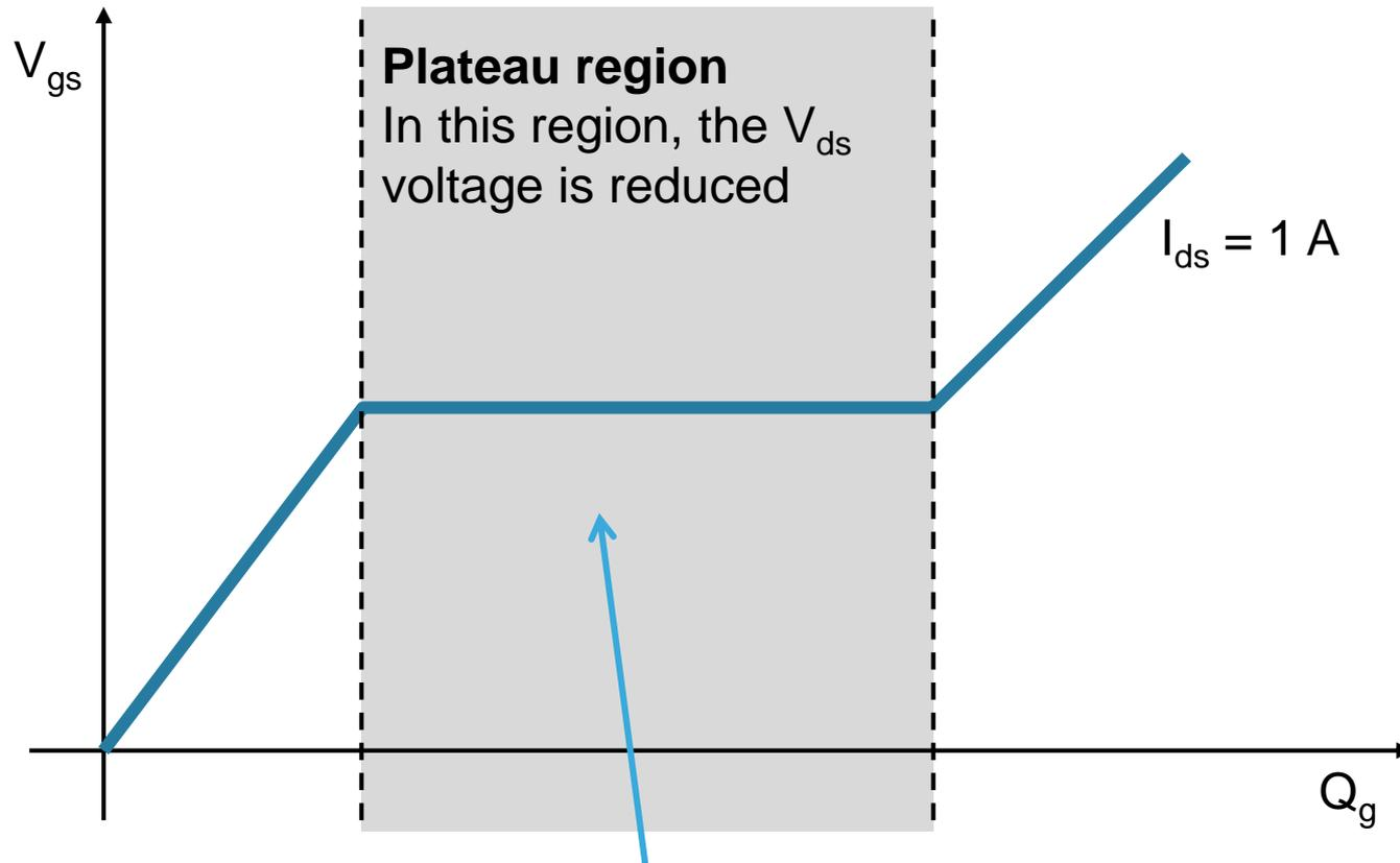
By charging the gate with a controlled current in this region, the slew rate of the power stage will be constant.
