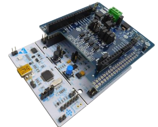
X-NUCLEO-OUT08A1 plugged on to a compatible STM32 Nucleo board
