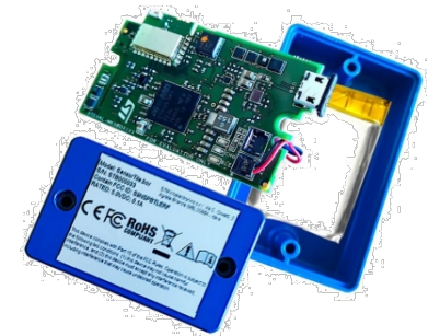
Ready-to-use box kit with wireless IoT and wearable sensor platform STEVAL-MKSBOX1V1
