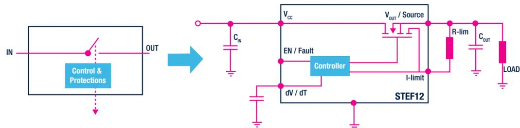
When an overload or short-circuit condition occurs, the eFuse limits the current to a pre-defined safe value. When an overvoltage condition occurs, the eFuse clamps the output voltage to a safe level, thus protecting the load from abnormalities caused by malfunctioning power supplies.
