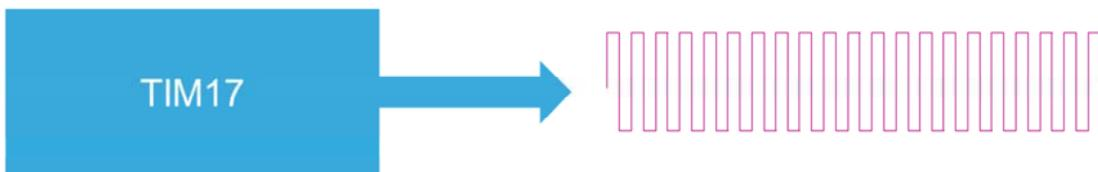
Timer 17 generates the carrier frequency for the remote control protocol used in the application.
