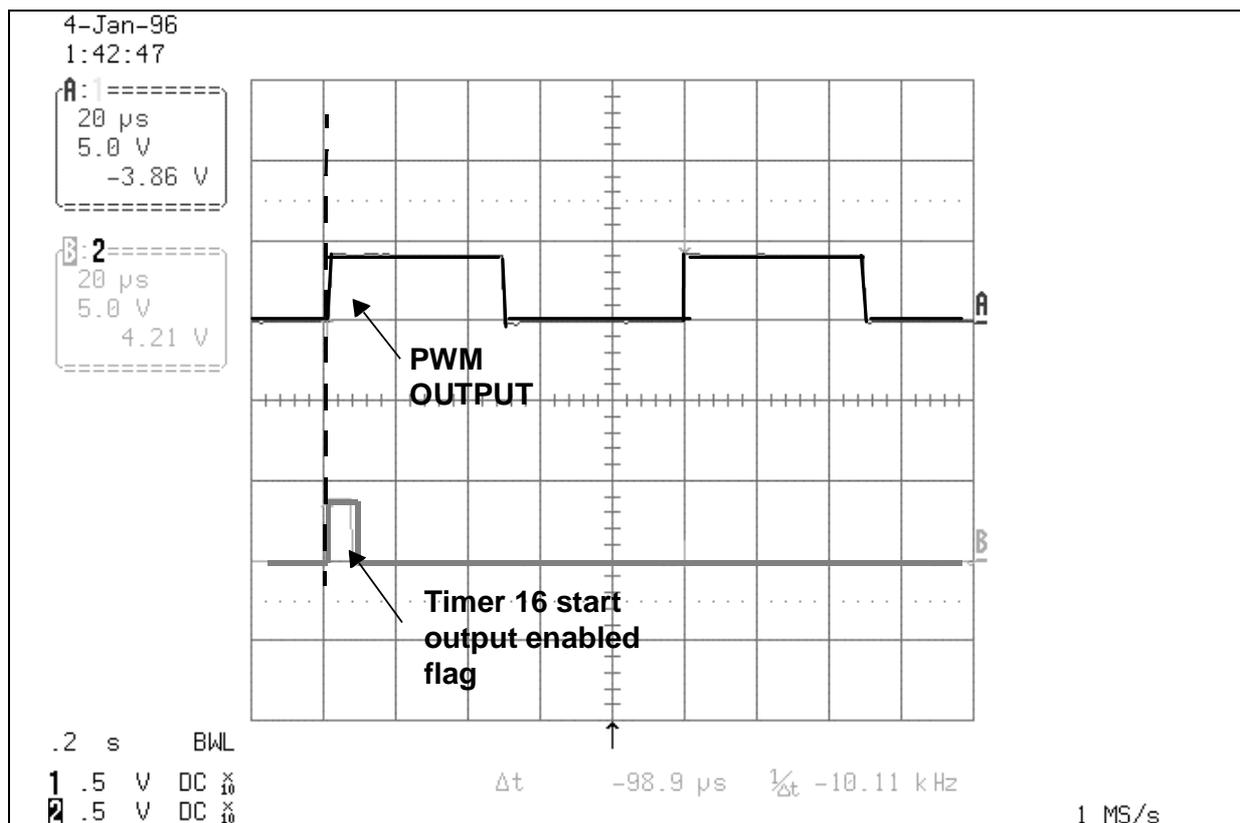
We can see in Figure 3 that the OCMP1 pin outputs a high state directly after starting the PWM signal. This avoids losing a PWM cycle in applications where an immediate high state is required.
