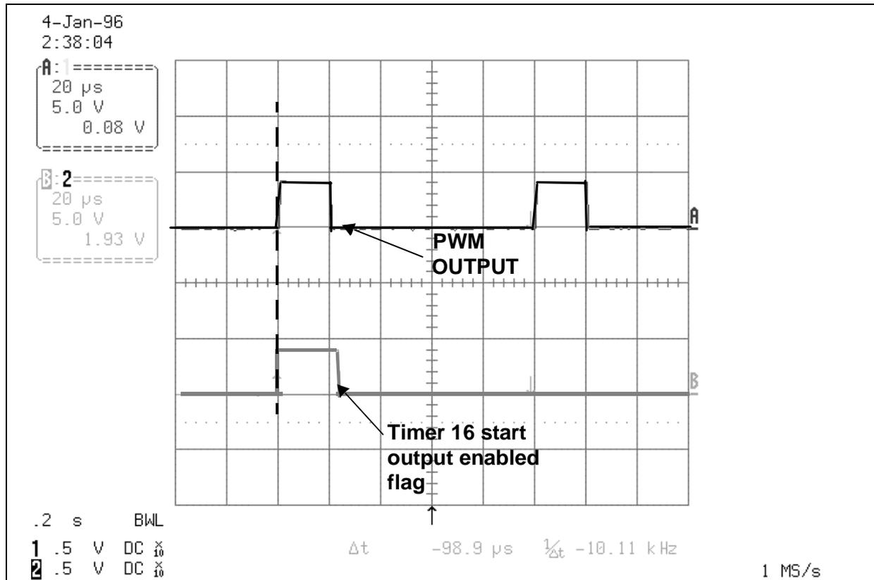
We can see on this figure that the OCMP1 pin outputs a high state immediately after starting the PWM signal with the 16 bit timer. This will avoid wasting PWM cycle for applications where an immediate high state is needed.
