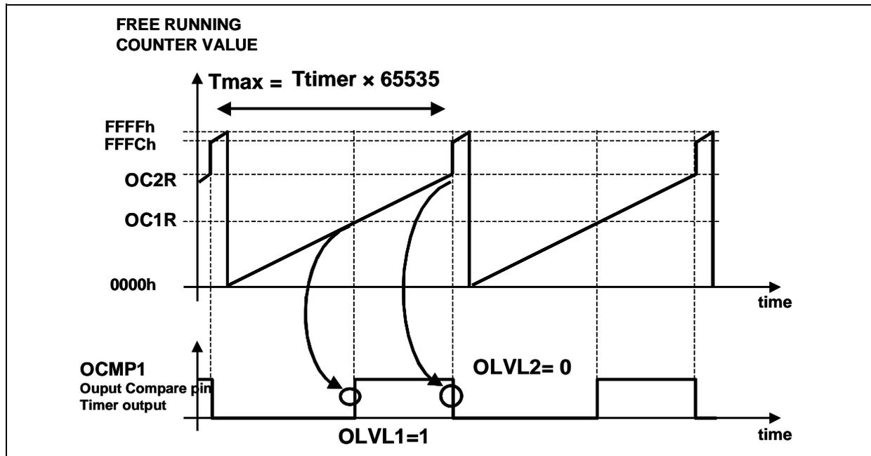
In this case, the timer A is also initialized at 10KHz with a 1MHz timer clock.
