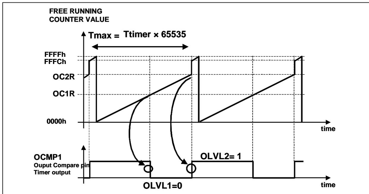
When the counter reaches the OC2R register value, the value of OLVL2 is applied on the OCMP1 pin (=1 in this case). When the counter reaches the value of the OC1R register, the value of OLVL1 is applied on the OCMP1 pin (=0). The formulas needed to compute the values to be put in OC2R and OC1R registers are in the 16-bit Timer chapter of the ST7 datasheets. As the 16-bit Timer is reset at FFFC, the formulas are:
