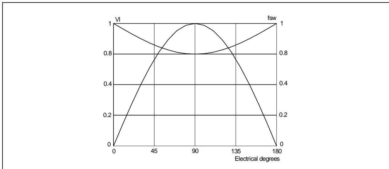
Considering the above mentioned points, to make a reasonable comparison with an equivalent fixed frequency PFC application in terms of EMI, it is recommended to modify the starting frequency (oscillator).
