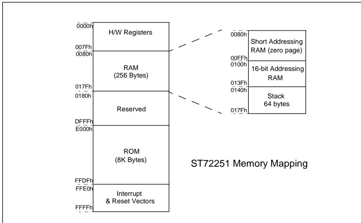
The ST7 RAM and ROM locations are addressed and read in the same way. For the ST7 core fetching and decoding instructions located either in RAM or ROM, take the same time, there is no limitation executing code in RAM.
