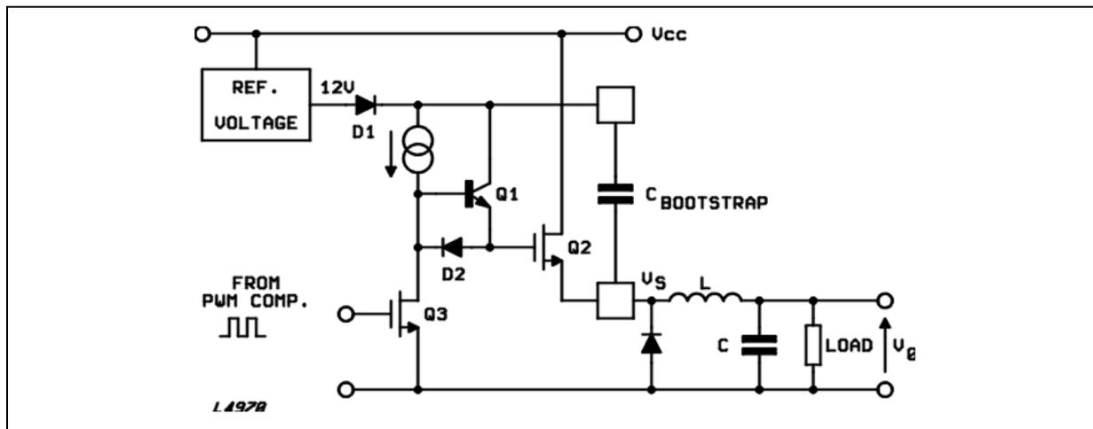
The five devices of L497X family differentiate each other only for the level of current protection, while the control part is the same and power device area is the same to guarantee low power dissipation also for low current versions in DIP package.
