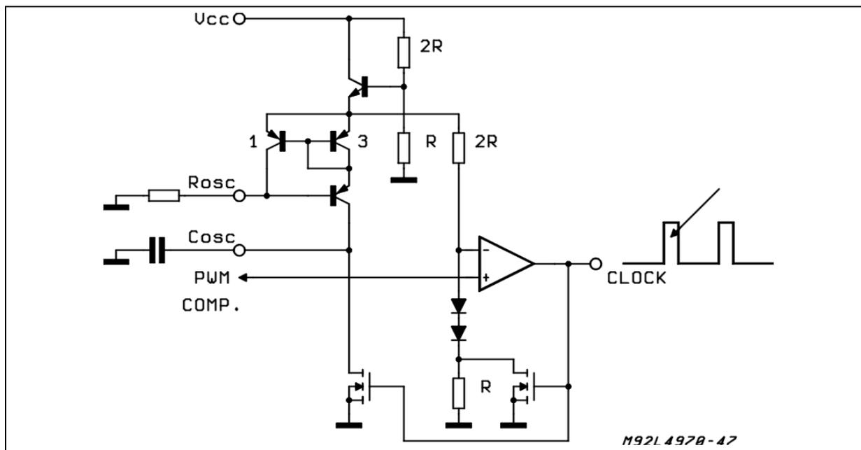
From fig.5 it is shown that the duty cycle changes due to the ramp increase when  $V_{cc}$  increases. The error amplifier output doesn't have to change to keep the loop in regulation. This feature increases significantly the line regulation performance.
