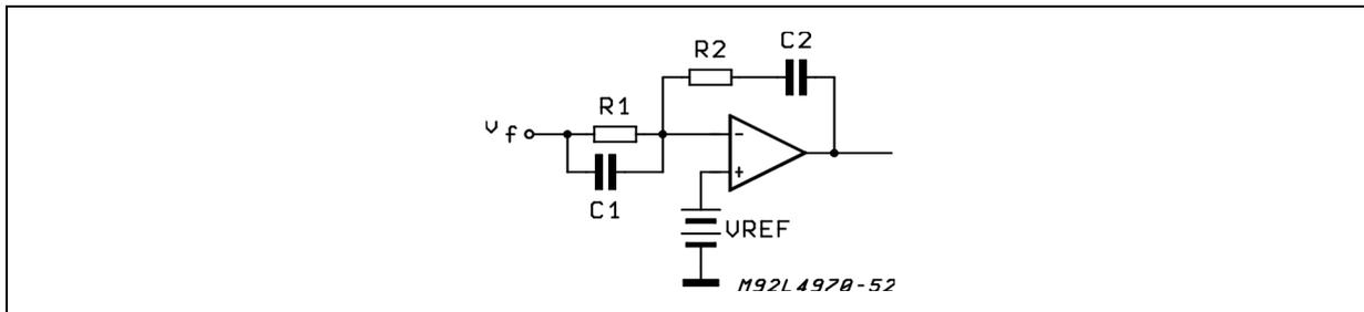
Such a configuration introduces a low frequency pole and two zeros  $Z_1 = 1/2\pi R_1 C_1$  and  $Z_2 = 1/2\pi R_2 C_2$ . Note that due to the high output impedance it is present also a second pole  $p_2 = g_m/2\pi C_1$ . Usually it is better to use the highest possible value for  $R_1$ , to have a low value for  $C_1$  in such a way to put  $p_2$  at the highest frequency. Limitations to  $R_1$  value are put by offset voltage due to opamp. input bias currents.
