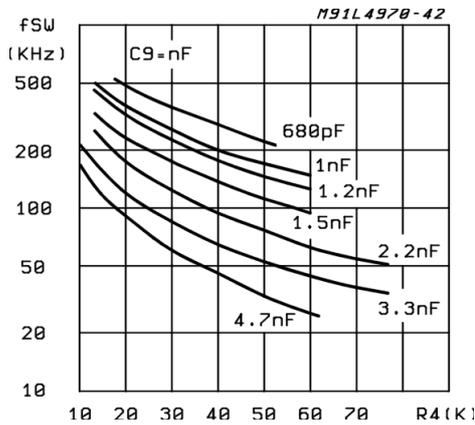
**Figure 7. Switching frequency vs. Rsc (L4972A/74A).**
