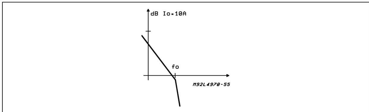
The system requires that DC gain is maximum to achieve good accuracy and line rejection. Beyond this a bandwidth of some KHz is usually required for a good load transient response. The error amplifier transfer function must guarantee the above constraints. A compensation network that could be used is shown in fig.19.
