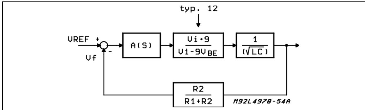
Consider the block diagram of fig.17, representing the internal control loop section, with the application values:
