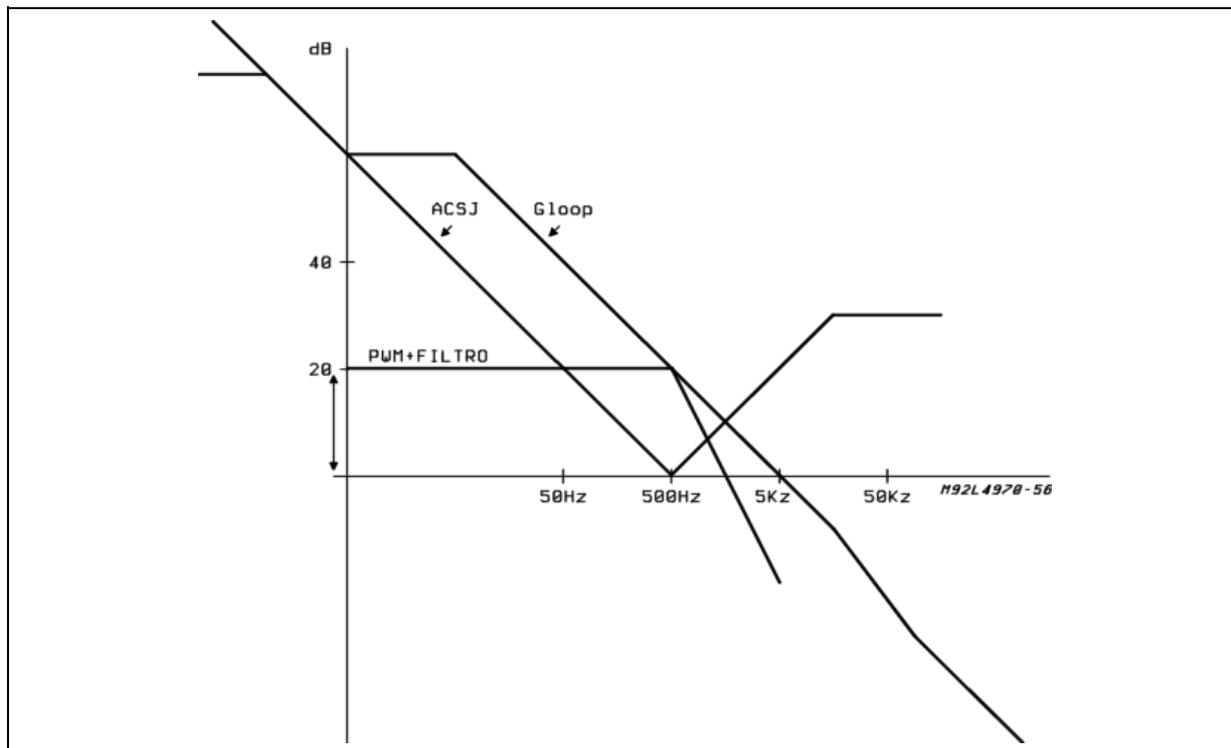
The criterium is to define Z1, Z2 close to the resonant pole of the output LC filter. The  $G_m/2PC1$  pole must be placed at a frequency at which open loop gain is below 0 dB axis (Fig. 20).
