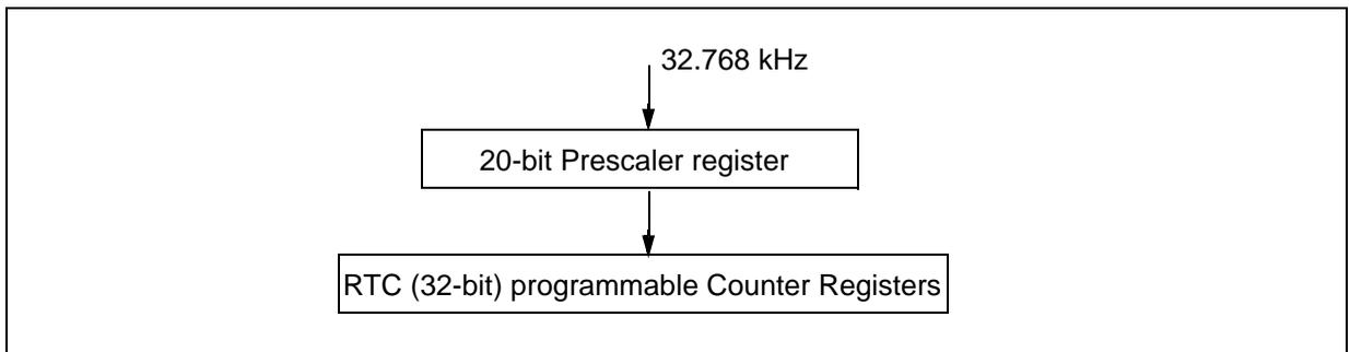
In this application, the RTC counter registers have to be incremented every second, this can be configured by using a prescaler value of 0x8000 (32768) to slow down the RTC clock from 32768 Hz to 1 Hz. This allows the RTC to keep time in seconds in the 32-bit counter.
