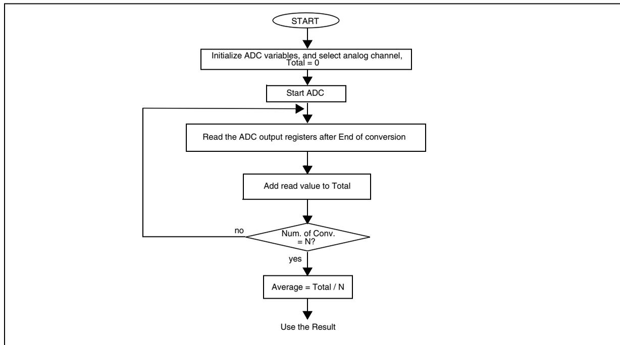
Table 4 is for reference only, representing the relation between the number of samples and the accuracy. After 25 samples, it shows an LSB accuracy of 2. The number of samples to choose depends on the application (noise level and timing) as these two are directly proportional. The disadvantage of having too many samples is that it takes more time to convert the data.
