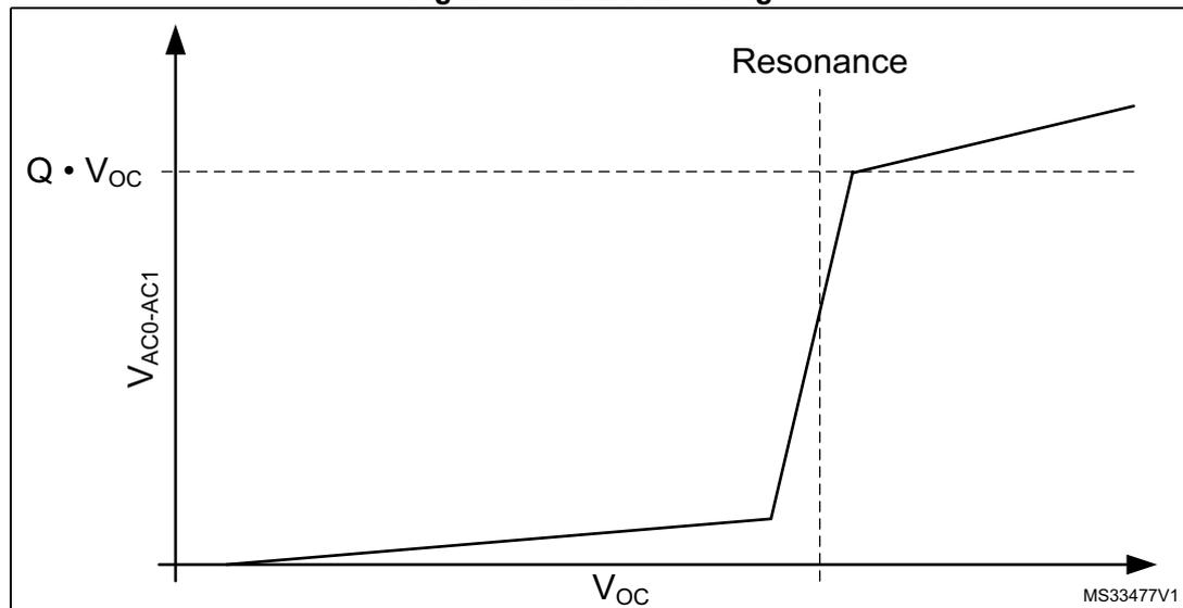
As  $V_{OC}$  increases, a sharp increase of  $V_{AC0-AC1}$  occurs when the serial capacitance of the M24LR reaches a value that satisfies the resonance condition
