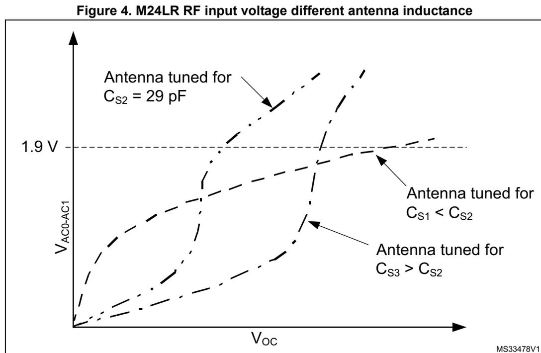
As shown in [Figure 4](#), the minimum RF voltage  $V_{OC}$  for which  $V_{AC0-AC1}$  is above  $1.9 V_{PEAK}$  (and consequently maximum distance at which the M24LR can operate) is reached for an antenna inductance  $L_A$  designed for  $C_S = 29$  pF.
