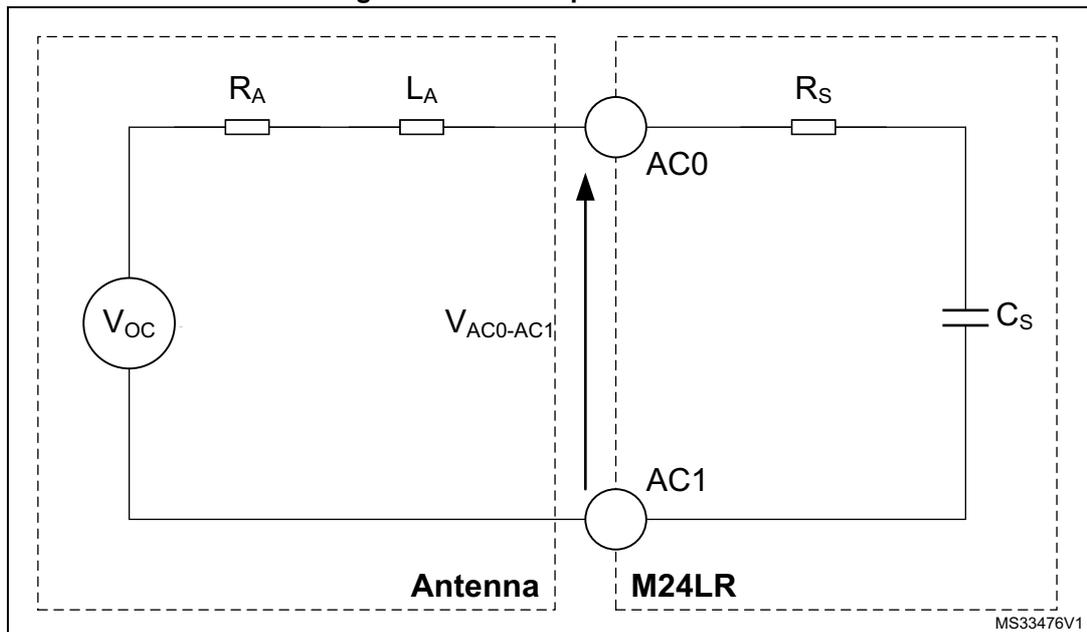
$V_{OC}$  represents the open circuit voltage available from the antenna. When a sinusoidal magnetic field (H) flows through the M24LR antenna, the open circuit voltage amplitude ( $V_{OC}$ ) can be determined using the following equation.
