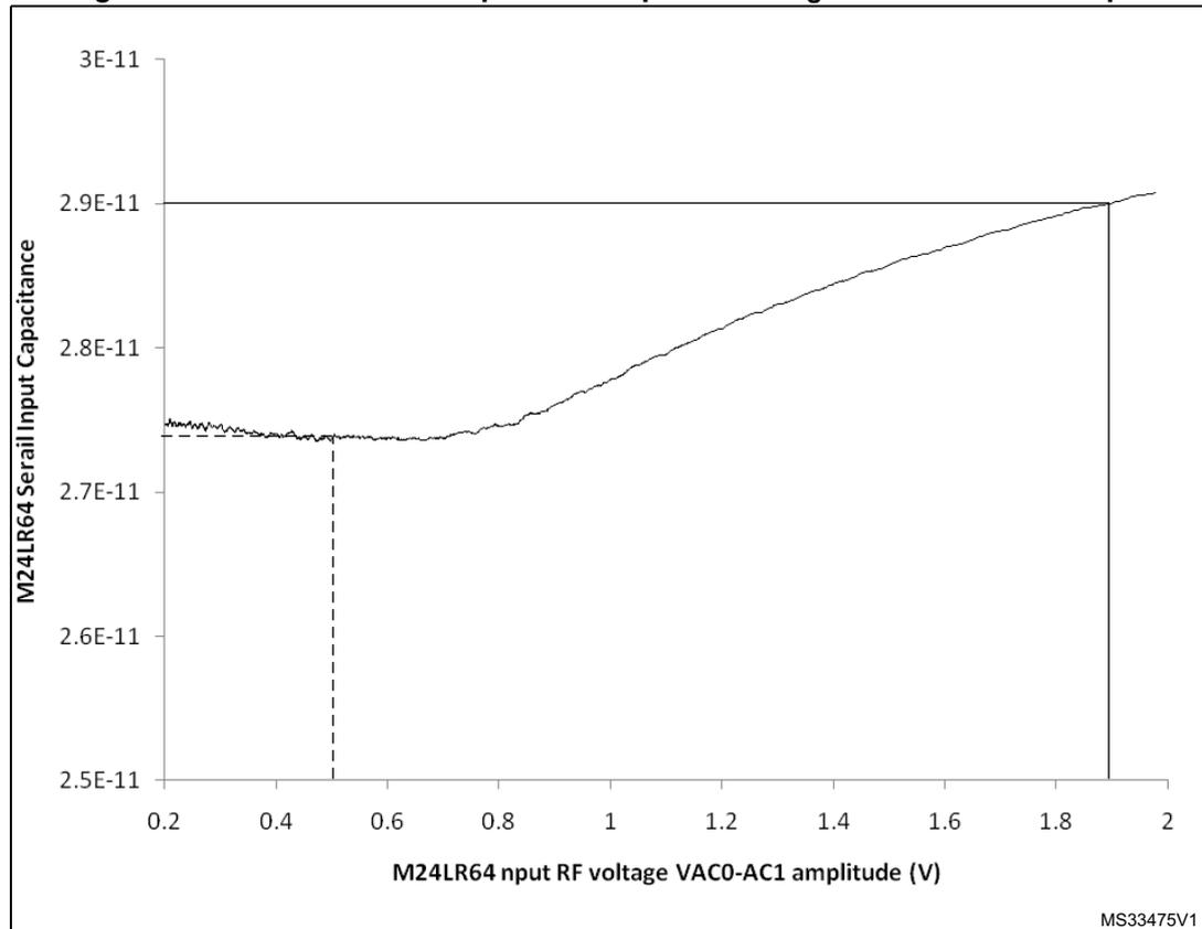
The dotted line in Figure 1 corresponds to the voltage level (0.5 V) at which the serial capacitance ( $C_S$ ) of the M24LR series is measured in production and specified in the datasheet (27.5 pF).
