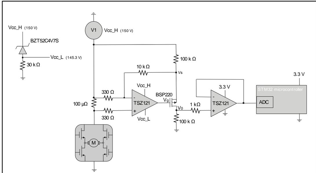
The maximum current drawn by the motor control is 100 A. So, for a 0.1 mΩ shunt resistor, the maximum  $V_{sense}$  is 10 mV. The maximum output voltage is dependent on the  $V_{sense}$  voltage, and the resulting output current flowing across  $R_4$ . As this current is treated by the ADC of the STM32 microcontroller, the maximum output voltage,  $V_o$ , must not exceed 3.3 V.
