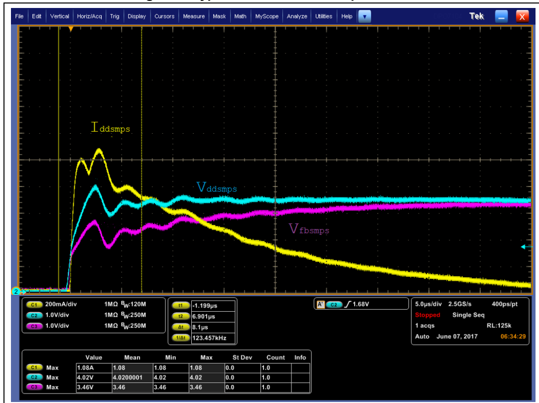
Figure 4. Typical inrush current at power-on
