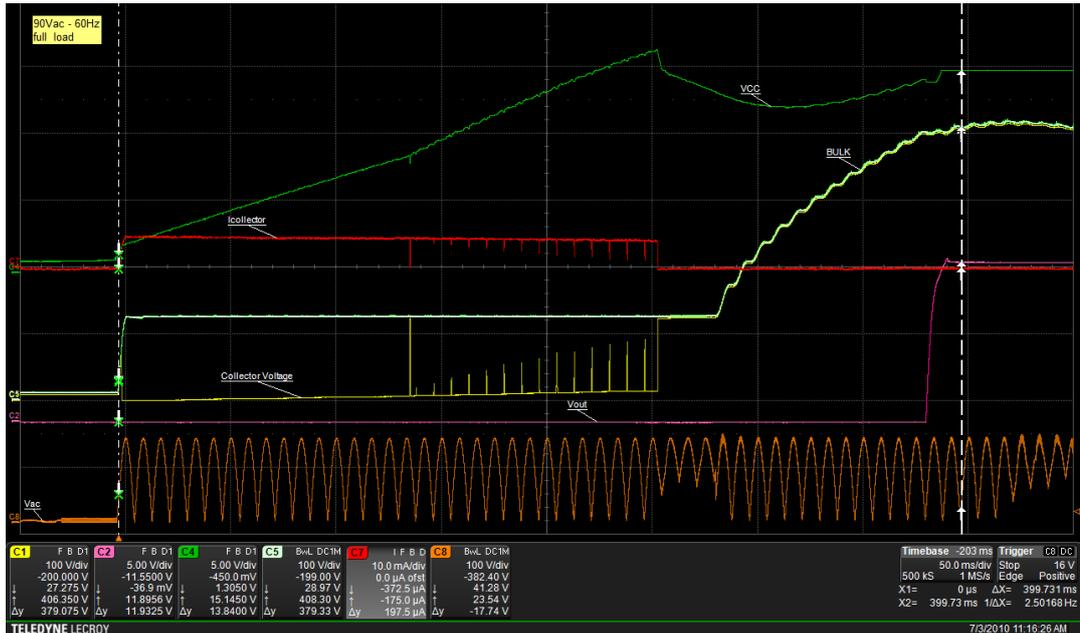
Figure 8 – 90Vac 60Hz full load startup with start-up booster
