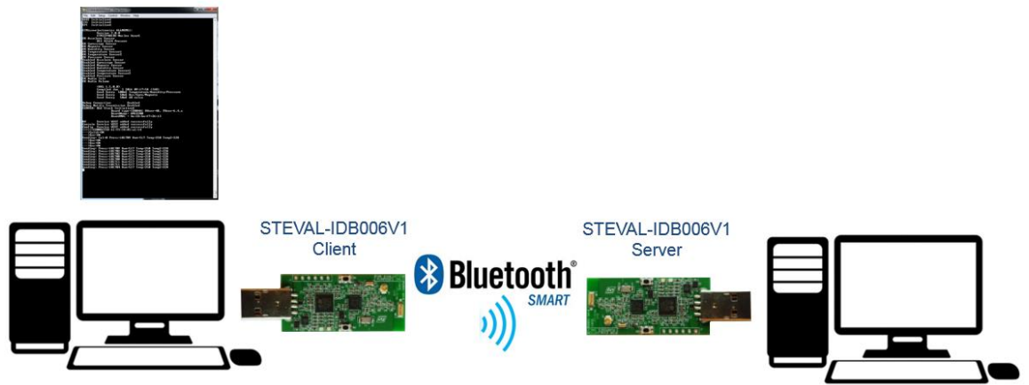
Figure 1: BLE Chat system setup
