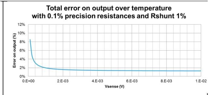
Figure 3: Total error assuming 0.1% resistances with Rshunt 1%
