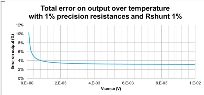
Figure 2: Total error assuming 1% resistances with Rshunt 1%
