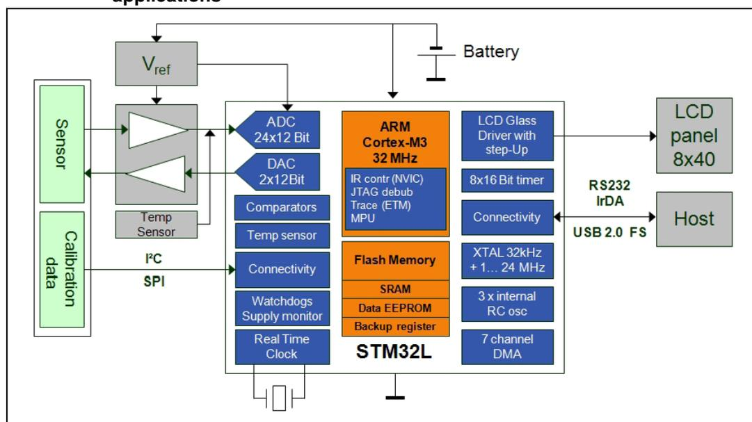
The proprietary mixed signal EEPROM technology used in the STM32L permits to integrate many of the components on a single chip leading to a reduction of the bill of material, and simplifying the power consumption and battery management.
