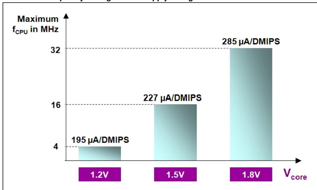
The idea is to keep the STM32L running at  $V_{core}=1.2$  V and to switch to a higher performance range only when the microcontroller needs to perform a specific task in a
