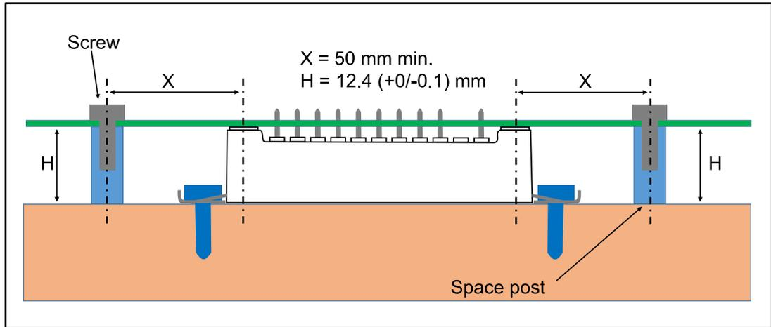
Figure 13: "Heat sink mounting" shows the overall assembly procedure when space posts are used. First the PCB with the modules is placed onto the heatsink (a). Then the modules are fastened to the heatsink through the screw clamps (b). Finally the PCB is fixed on the space posts.
