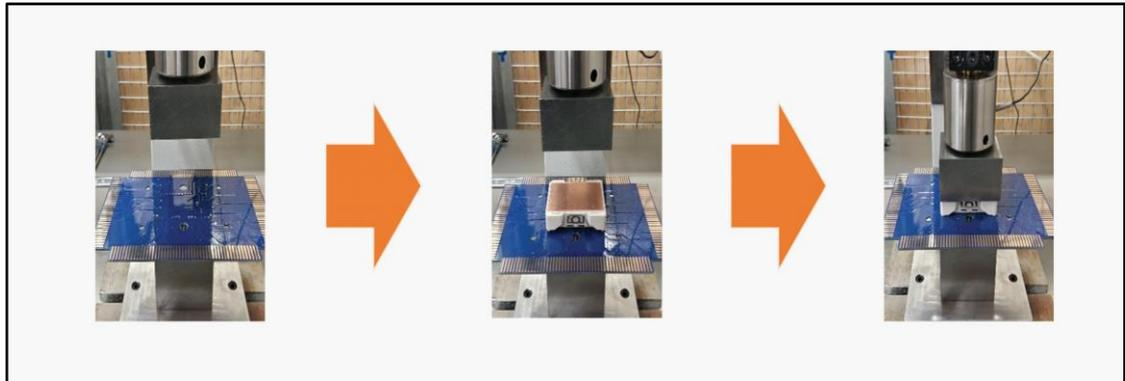
Generally, a module can be pressed in until the stand-offs on the four corners of the module touch the PCB.
