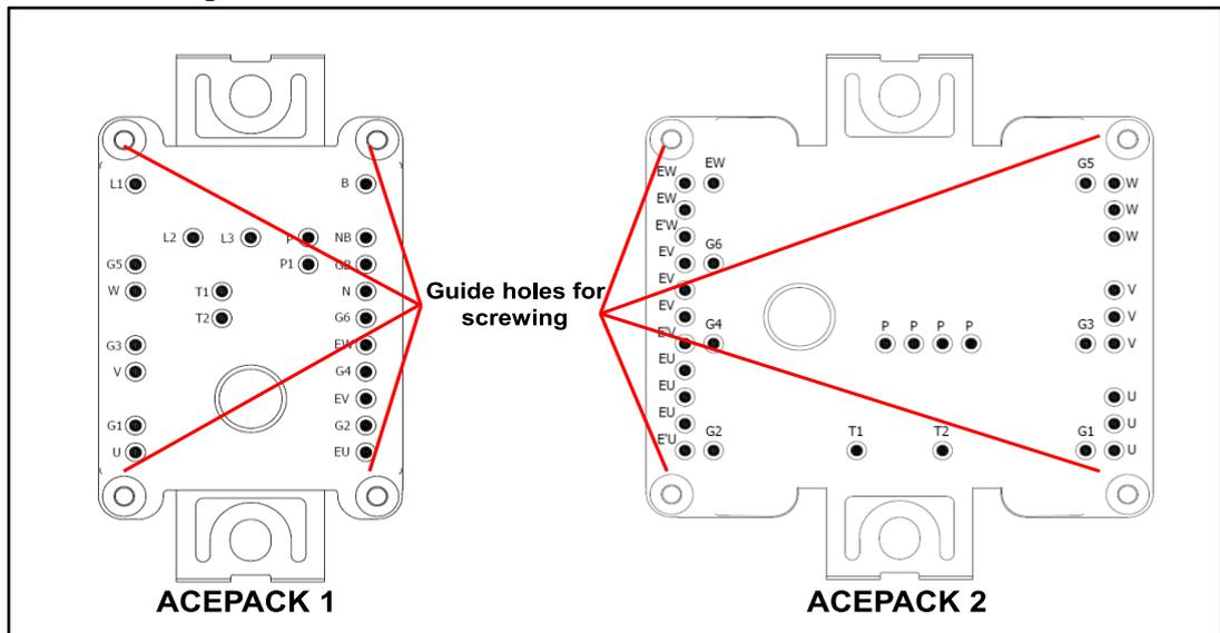
After the PCB mounting process, it is recommended to fix the PCB to the module with screws to ensure reliable contact. If an air gap remains between the module stand offs and the PCB, do not screw to avoid PCB bending. The figures above show the details for screwing the module. The effective length of a screw excluding the PCB thickness should be 4.0-8.0 mm. Screwdriver speed lower than 300 rpm and screwdriver torque  $0.4 \text{ Nm} \pm 10\%$  is recommended.
