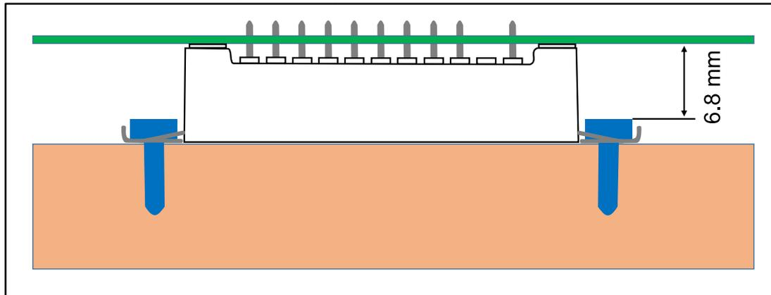
The minimum clearance distance between the screw and the PCB depends on the screw itself. The distance is 6.8 mm with a hexagon socket head screw according to DIN 912, a washer according to DIN 125 and the clamp, see [Figure 14: "Air path between clip and PCB"](#).
