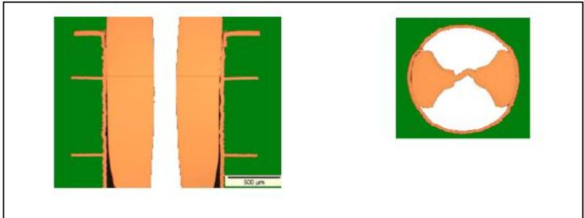
A module that has been pressed in and then pressed out again can no longer be pressed in again. Instead, the module can only be attached to a new printed circuit board by soldering. The plastic deformation of the press-fit zone does not permit further press-fit processes.
