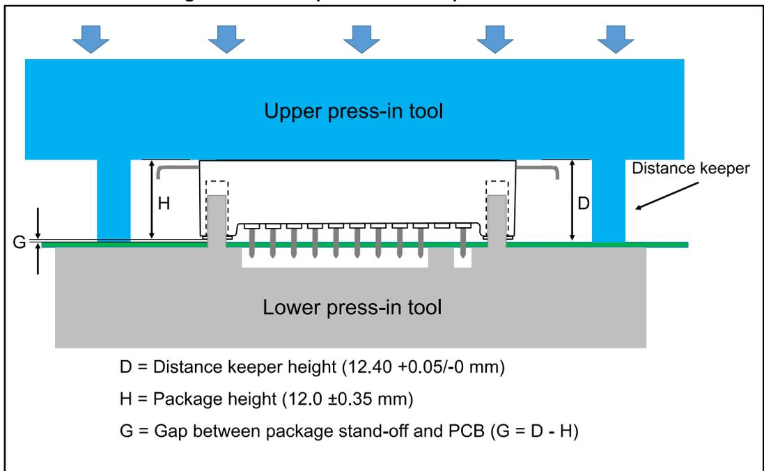
During the process, once the distance keeper contacts the surface of the PCB, the press-in force rises and the press-in process can be stopped, thus preventing direct contact
