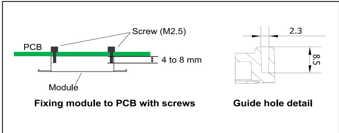
Figure 8: Guide hole for the screws in ACEPACK 1 and ACEPACK 2
