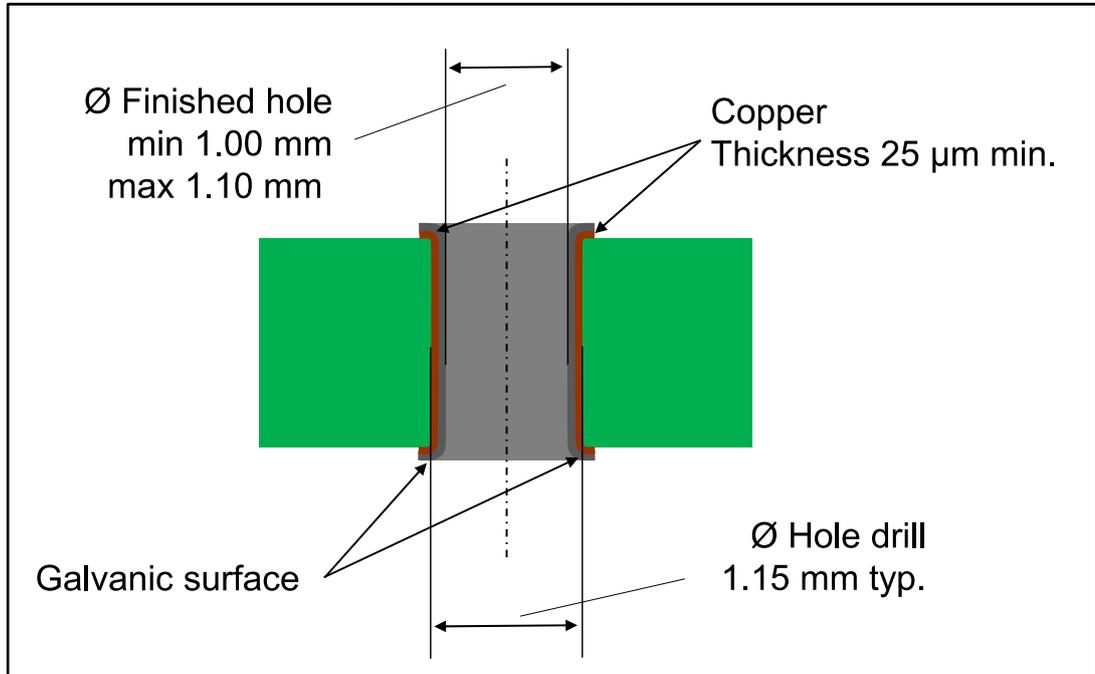
An adequate design of the plated through holes (PTH) of a PCB is essential to obtain good quality press-fit connections. If the finished hole diameter of the PTH is too small, the press-in force through the plated hole may be too high and cause mechanical damage to the pins and the PTH. If the finished hole diameter is too large, it may not form a reliable connection with the pin.
