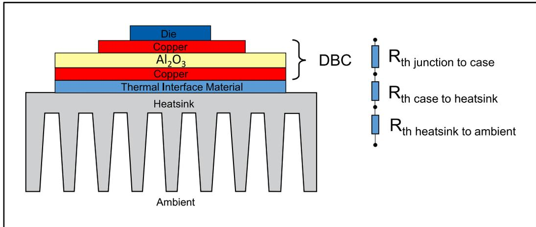
Proper contact between the module substrate and the surface of the heat sink is crucial for managing the overall thermal efficiency of the system. Thermal Interface Materials (TIMs) are thermally conductive materials used to allow proper matching of the two surfaces and improve heat transfer.
