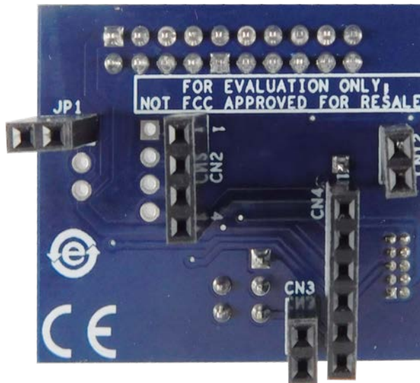
Figure 6. STEVAL-UKI001V1 bottom view
