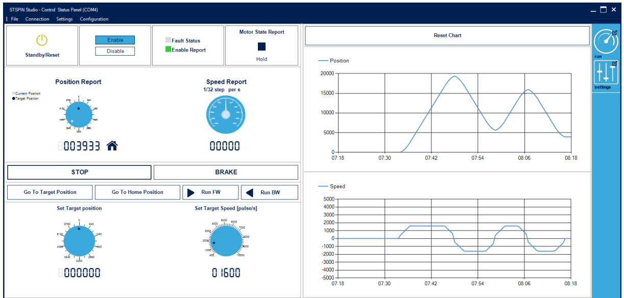
Figure 9. Stepper control with run panel
